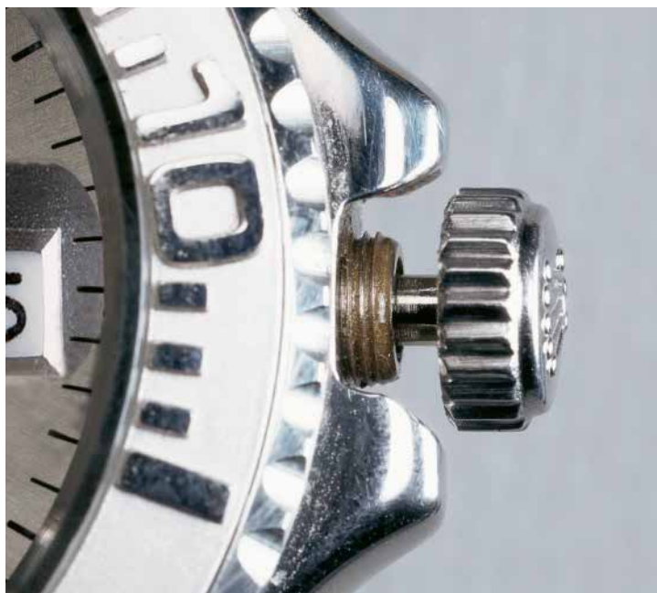
Clearly different: you can search the fake's crown for the wide-diameter tube and insulating ring, but you won't find them.
