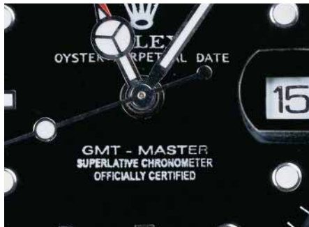
Gotcha! The word “superlative” is poorly printed on the dial of the fake (left).
