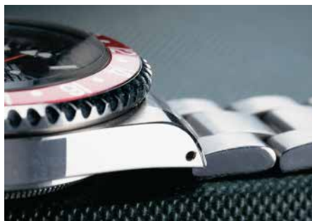
Typically fake: the hole (left) for the crosspiece hasn't been drilled cleanly.
