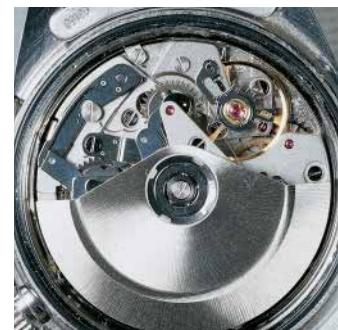
Inside the imitation Daytona: a Valjoux 7750, rebuilt to support a tri-compax display.
