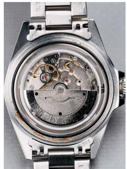
Miyota movement, plastic movement-holder ring, rust around the rim: this $50 fake is not a pretty sight.
